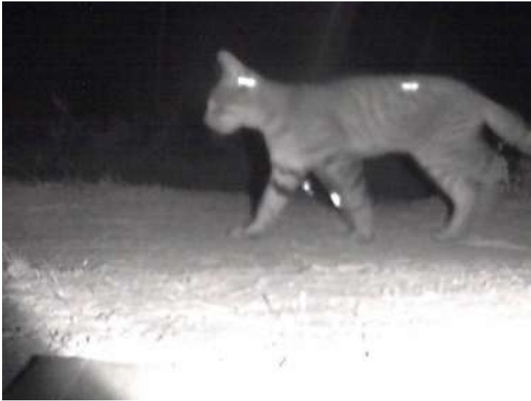
Figure 2. A feral cat from the Olympic Dam trial showing the activation sensors (revealed through infra red camera) intercepting the head and rump of the cat and the bottom blocking sensor passing between the cat's legs at the point of firing.
