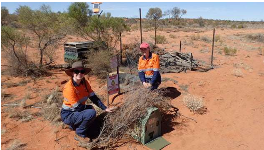
Figure 4. Felixers were set up across vehicle tracks adjacent to the fence where cat activity is highest. This site F33 is the same area that leg-hold traps have historically been used for cat control, either in the corral or elevated platform visible behind the Felixer.
