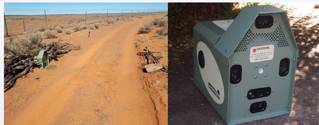
Figure 3. Felixers detect, distinguish and spray feral cats with toxic gel that is ingested by oral grooming
